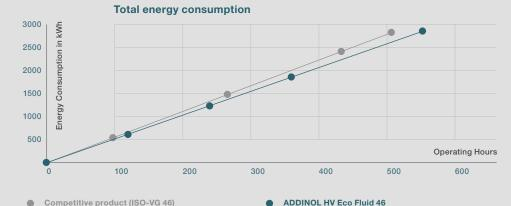
Energy Consumption (kWh) = **5.6192 kW** x operating hours
