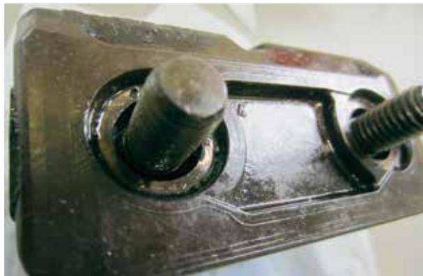
Clip without residues after 18,500 operating hours with ADDINOL Cliptec XHS 280
