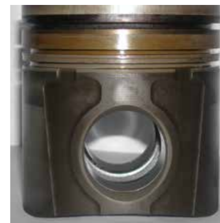
Aluminium piston with ring grooves MWM TCG 2016 V12
