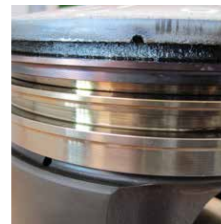
Steel piston with ring grooves INNIO Jenbacher J612 GS-F02
